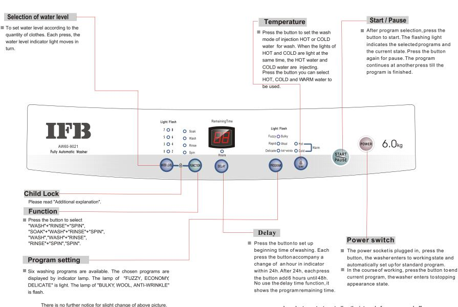
In order to protect controller, the interval of power on and off should be more than 30 seconds.
